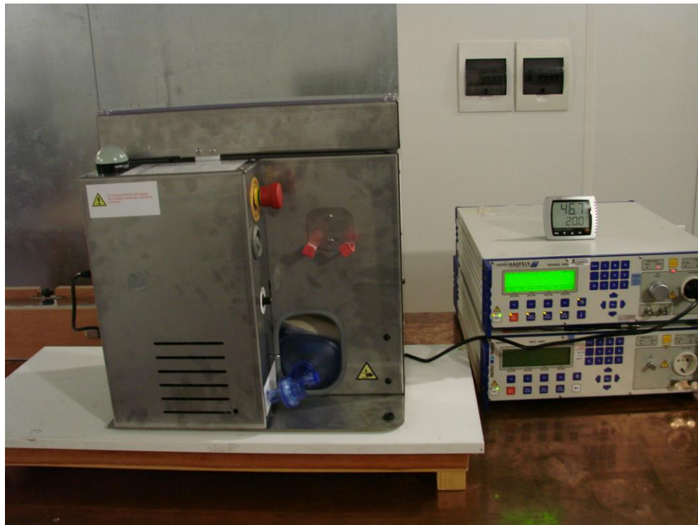
Figure 16 EUT Set-up for surges at AC power port
