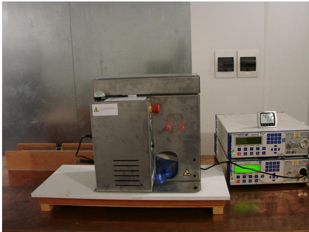
Figure 14 EUT Set-up for EFT at AC power port
